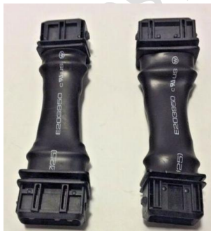
23. 5 Pin to 4 Pin 1.8T Audi ICM Delete Conversion Harness
